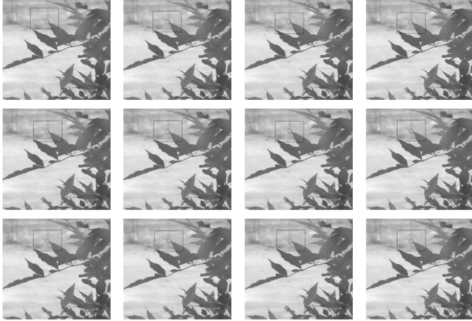
Fig. 5. Some frames of the tracking of the maximal cornerness point on an outdoor image sequence using SUSAN method.
